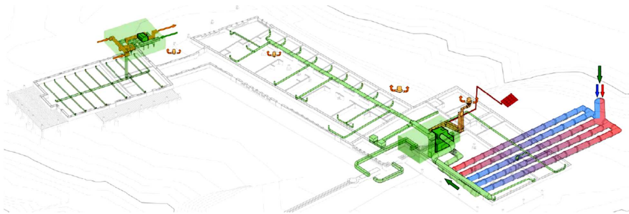
Figure 30. Earth duct inlet and outlet air 38
