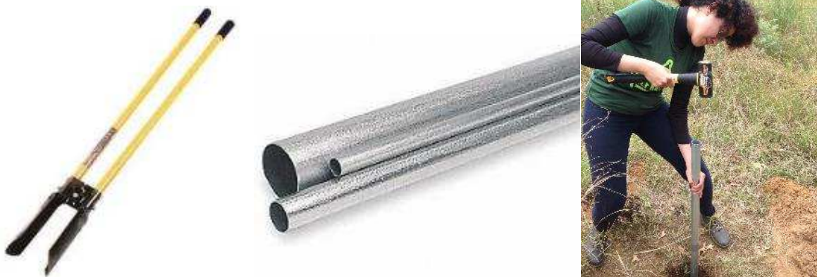
Figure 98. Hole Digger, Conduit
